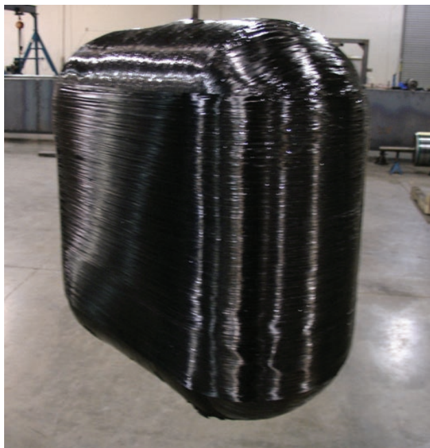
FIGURE 3. Prototype Filament Wound "Pillow" Conformable Pressure Vessel Segment
