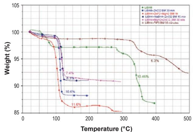
**FIGURE 2.** SDT of thermal decomposition profiles  $\text{LiBH}_4$ ,  $\text{LiBH}_4 + \text{ZnCl}_2$  ball milled 30 min,  $\text{LiBH}_4 + \text{ZnF}_2 + \text{MgH}_2$  ball milled 1h,  $\text{LiBH}_4 + \text{NaBH}_4 + \text{ZnCl}_2$  ball milled 15 min,  $\text{LiBH}_4 + \text{MgH}_2 + \text{ZnCl}_2$  ball milled 30 min and  $\text{LiBH}_4 + \text{TiF}_3$  ball milled 30 min.
