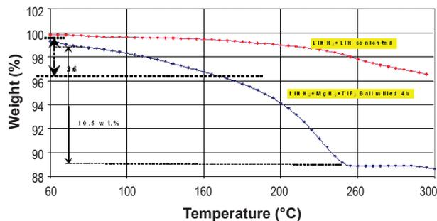
**FIGURE 4.** Thermogravimetric analysis curves for the plain LiNH<sub>2</sub>/LiH and Ti-doped/MgH<sub>2</sub> ad-mixed LiNH<sub>2</sub>.
