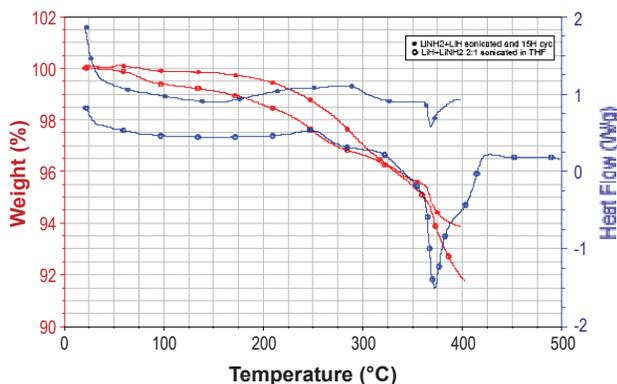
**FIGURE 3.** TGA and DSC profiles of LiNH<sub>2</sub>/LiH before and after 15 H-cycles.
