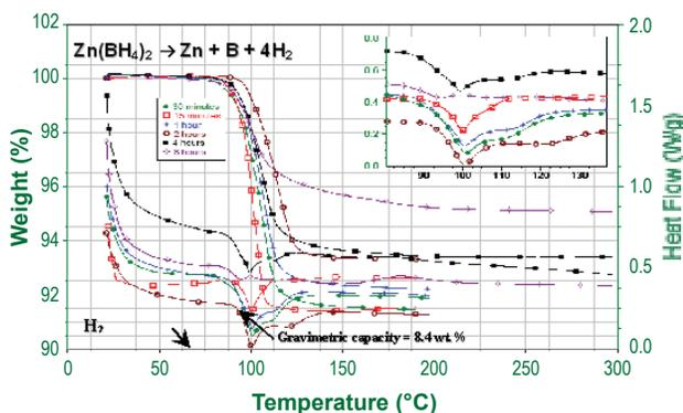
**FIGURE 1.** SDT of thermal decomposition profiles of  $\text{Zn}(\text{BH}_4)_2$  with different milling durations, 30 minutes, 1h, 2h, 4h, 8h.
