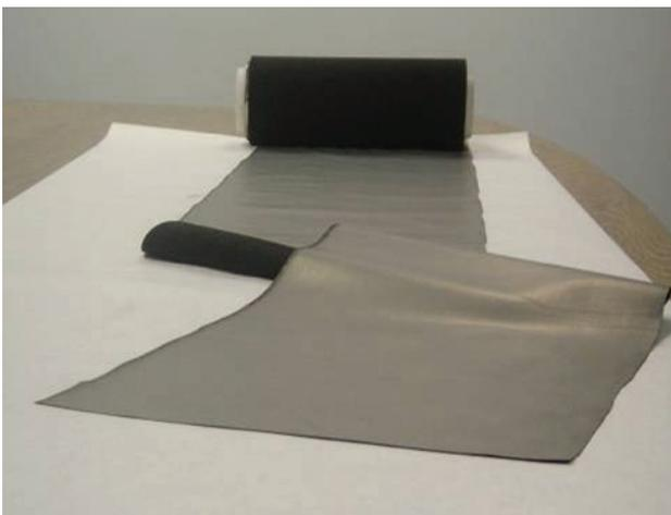
**FIGURE 1.** Roll-to-Roll Ion Beam Coating - Pt on ELAT GDL, Standard Gradient, 0.08 mg/cm<sup>2</sup>, 30 linear meters, Pt variation < +/-3%
