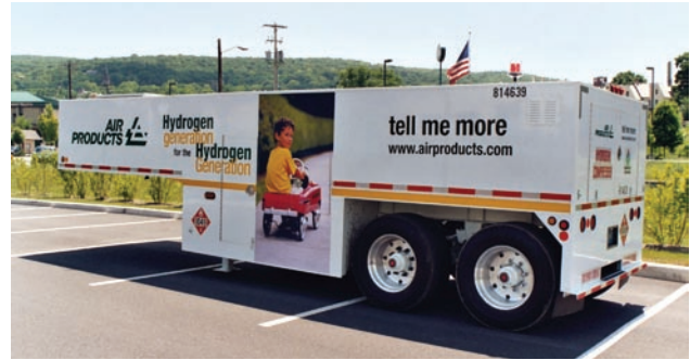
FIGURE 3. Air Products HF-150 Hydrogen Fueler
