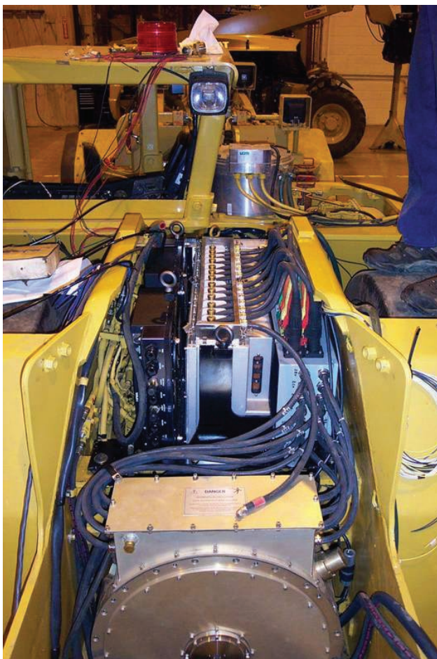
FIGURE 6. Traction Motor and Control
