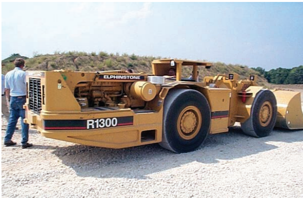
FIGURE 1. Diesel-Powered Mine Loader
