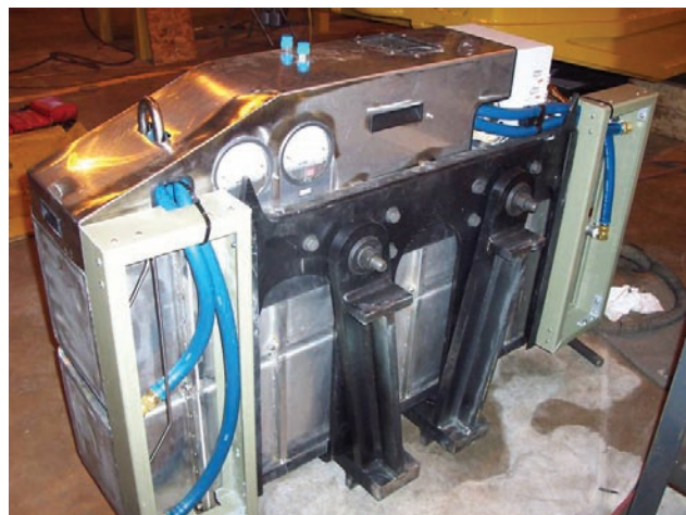
FIGURE 5. Metal-Hydride Storage Module
