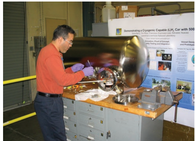
FIGURE 2. New Design for Insulated Pressure Vessel
