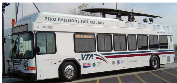
FIGURE 1. The Buses at VTA use a Non-Hybrid Fuel Cell System Developed by Ballard Power Systems
