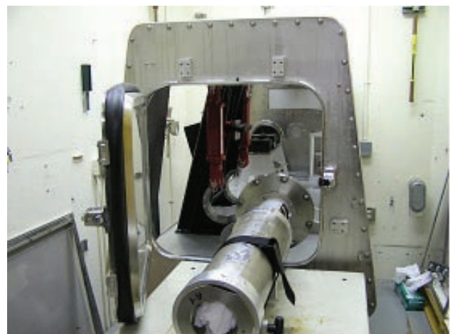
FIGURE 4. Glove Box for Preparing Crack-Growth Specimens in Low-Oxygen Environment
