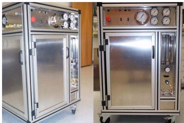
Figure 5. Mobile Demonstration Platform That Houses All System Components, Pumps, Valves, and Control System Functions of the InnovaGen™ Fuel Processor
