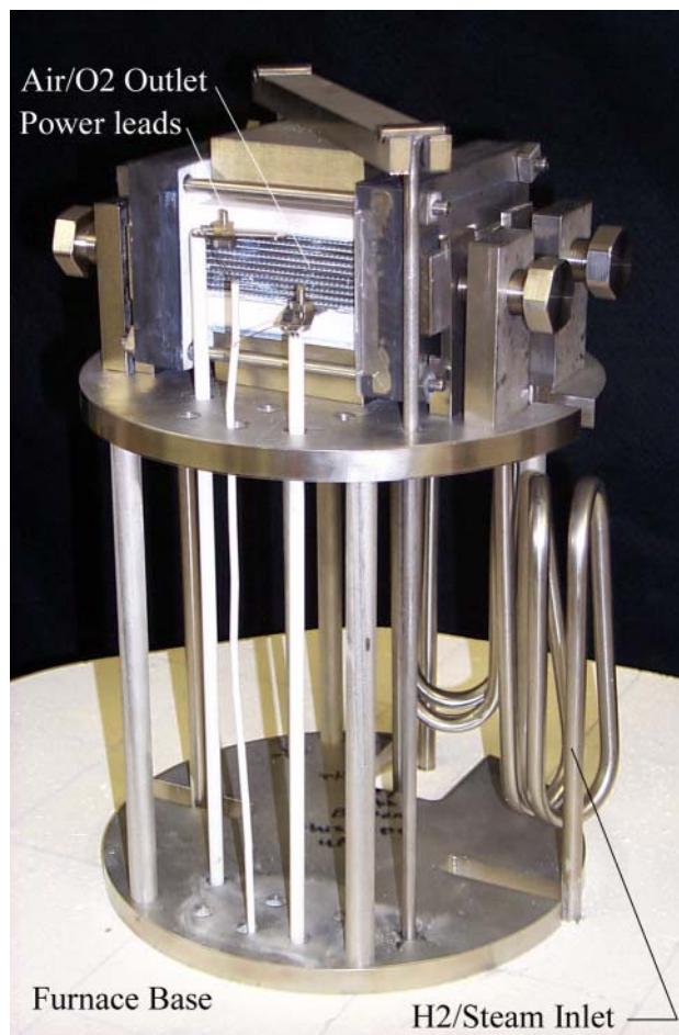
Figure 5. Ten-Cell Electrolysis Mounted for Testing at INEEL
