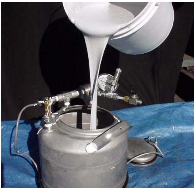
Figure 1. Lithium Hydride Slurry
