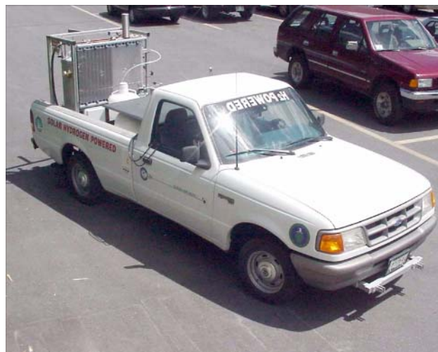
Figure 2. Laboratory Lithium Hydride Slurry Mixer System Mounting in a Hydrogen-Powered Pickup Truck
