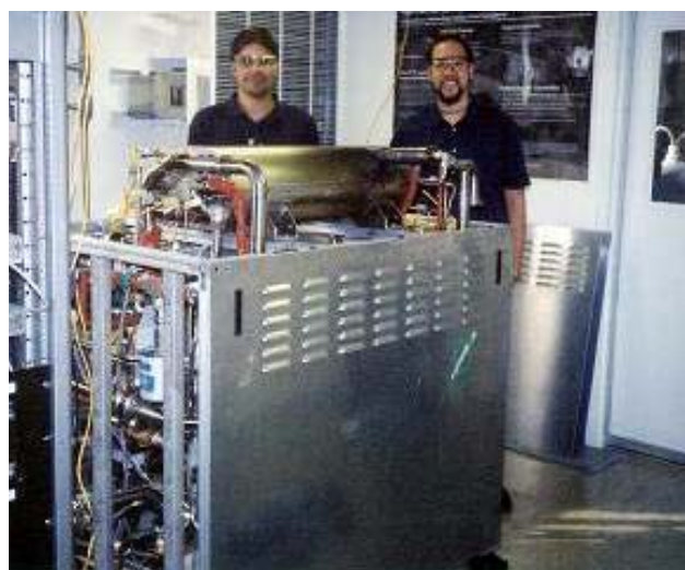
Figure 4. STAR Fuel Processor System Installed at Argonne National Laboratory
