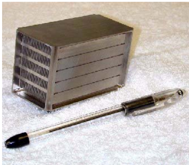
Figure 2. Differential-Temperature Section of the 2-kW e -Scale WGS Microreactor
