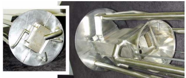
Figure 6. Recuperator/Mixer Assembly Delivered to ANL as Part of the FASTER Project (At left the mixer assembly can be seen at the exit. Hot reformate enters the round to square transition at right.)
