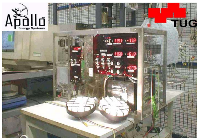
Figure 4. The TU-Graz/Apollo Alkaline Fuel Cell/Hybrid System with Ammonia Cracker (in the rear, heat-insulated)
