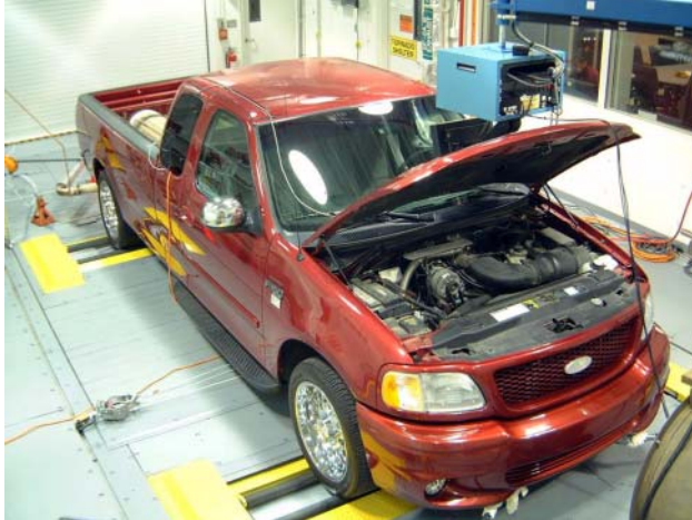
Figure 1. Ford F-150 Truck on Dynamometer at Argonne National Lab
