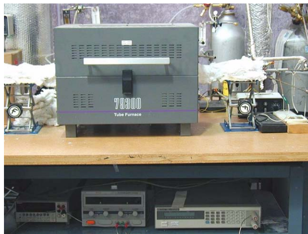
Figure 1. Picture of the SOFEC-SOFC Test Rig, Capable of Operating in Both SOFC and SOFEC Modes
