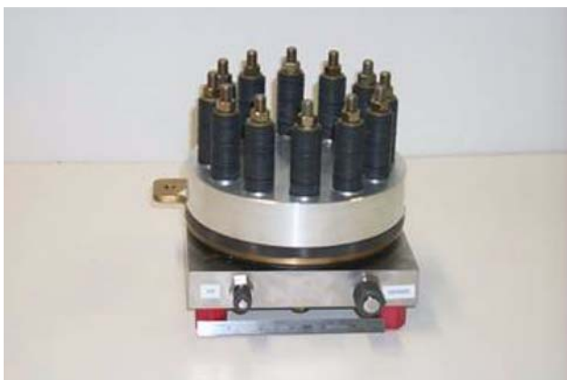
Figure 4. Photograph of PES Test Electrolyzer (80 cm 2 Active Cell Area)
