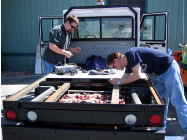
Figure 4. Conversion to a Fuel Cell Vehicle Taking Place at the Las Vegas Valley Water District
