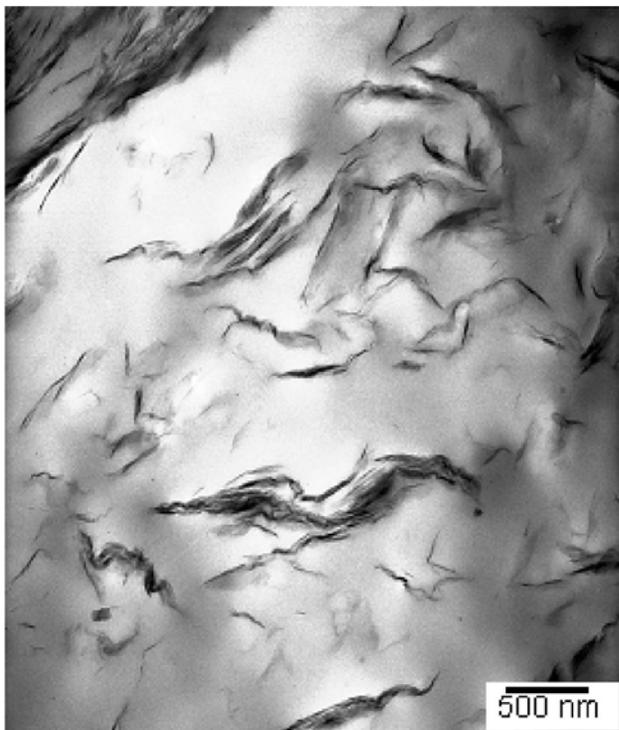
**Figure 2.** TEM Micrograph of PET/10% Clay Nanocomposite (The clay appears as dark ridges in the lighter-shaded PET. Some intercalation of the clay platelets is evident.)
