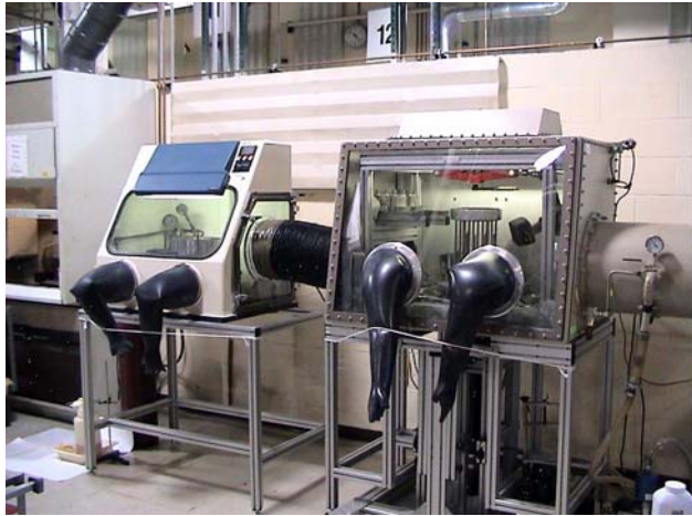
Figure 2. Dual glove box assembly used to fabricate CCHSS#1. The left hand glove box was used to fill the foam disks while the right hand box served as the loading station for the vessel which is mounted vertically and required an electrically driven press to drive the foam disks over the stainless steel tubes.
