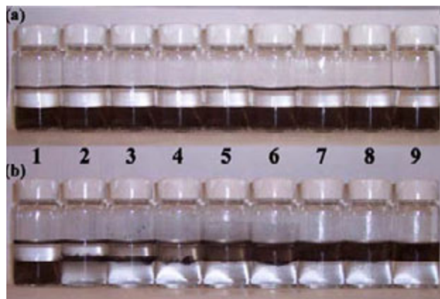
Figure 1. The effect of TOAB concentration on the extraction of SWNTs into an ethyl acetate phase. The solutions (a) before and (b) after extraction. The TOAB:SO 3 - ratios for vials 1 – 9 are 0, 0.15, 0.3, 0.45, 0.6, 0.75, 0.9, 1.0, and 2.0, respectively.
