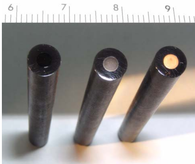
Figure 3. A Series of Glassy Carbon Disk Electrodes Depicting Steps in the Spontaneous Deposition Process (From left to right; uncoated, CS1 coated, and heavily gold deposited microelectrodes.)
