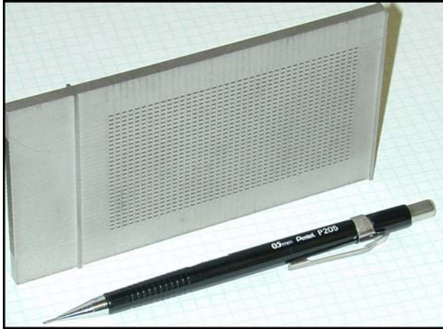
Figure 4. Micro-Channel Water Vaporizer for 5 kg/day System (This heat exchanger produces superheated steam from water feed in a single step with very low air-side pressure drop.)
