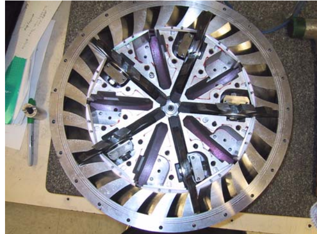
Figure 3. Primary Vanes with Improved Surfaces in Housings
