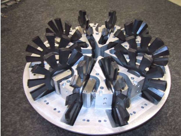
Figure 1. Secondary Rotors as Dynamic Valves in Housings
