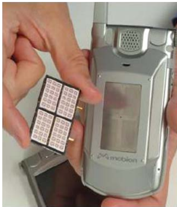
Figure 2. Rugged Fuel Cell Array and Fuel Cell Powered Device Demonstrator
