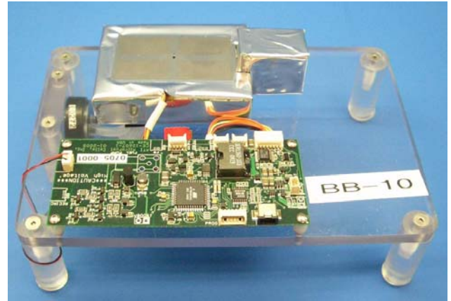
Figure 4. Breadboard Test Hardware – Cartridge not Shown
