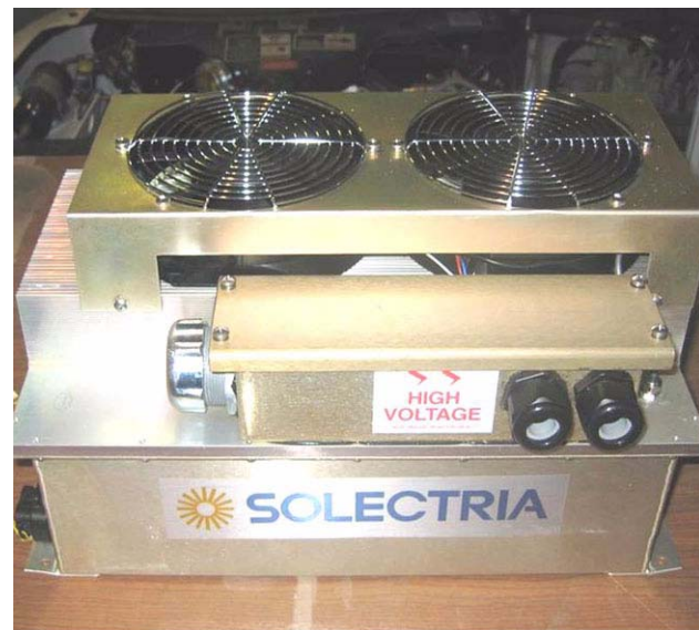
Figure 6. DC to AC Power Converter Used to Supply Power to the APU
