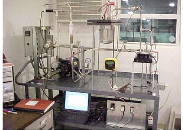
Figure 1. Dynamic Test Loop at the Dynalene Facility to Test Various Fuel Cell Coolants
