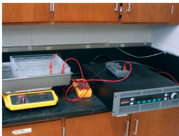
FIGURE 1. Pulsed DC Power Supply with Electroplating Bath for Electrodeposition of Porous Nickel
