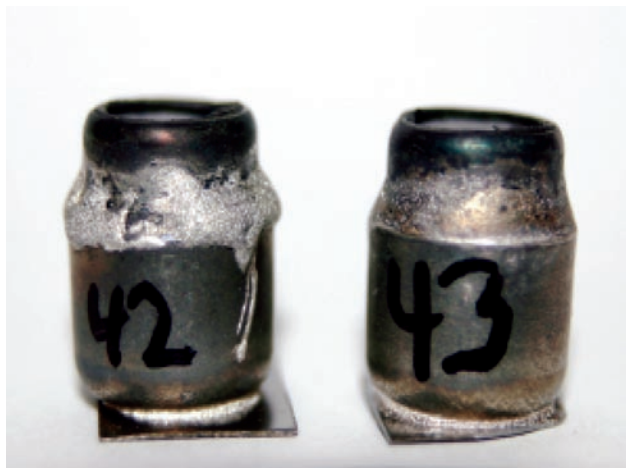
FIGURE 1. Successful Braze of Membrane Alloy to Stainless Steel
