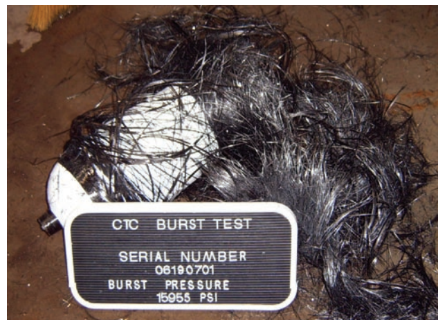
FIGURE 2. Type II COPV with Sidewall and Hoop Failure
