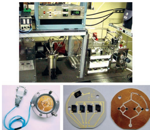
FIGURE 3. Flow system, 2 kpsi Parr reactor, and control electronics (top); four sample hotplate with one TCD hotplate PCB assembly (bottom right) and conflat flange mounted assembly (bottom left).
