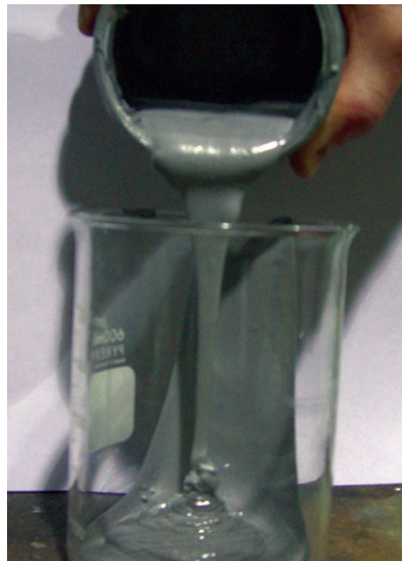
FIGURE 2. 70% MgH 2 Slurry Made From Milled Particles
