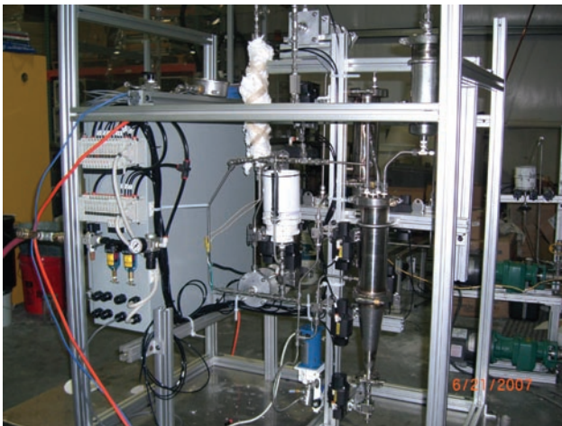
FIGURE 4. Model #4 MgH 2 Slurry Mixer Apparatus
