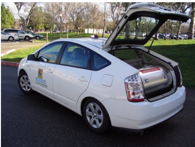
FIGURE 1. Cryo-Compressed Vessel Installed Onboard the Prius Hydrogen-Fueled Hybrid Vehicle
