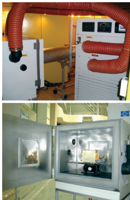
FIGURE 1. Photo of the freeze chamber installed inside the Neutron Imaging Facility (top). The sample chamber with 100\text{ cm}^2 cell inside is also shown (bottom). Windows on front and back are designed for neutron transmission and thermal insulation.
