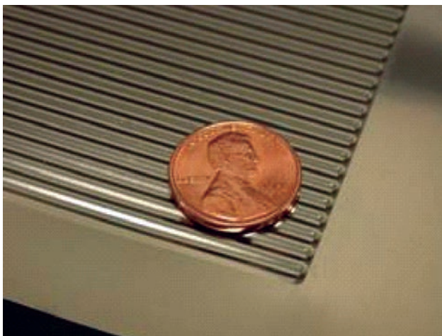
FIGURE 1. Stamped Metallic Bipolar Plate (After Reference 1, Courtesy of GenCell Corp.)
