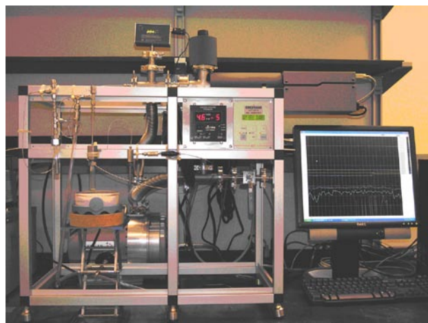
FIGURE 3. In-House Built for Measuring Kinetics and Purity of \text{H}_2 Evolution in Real Time
