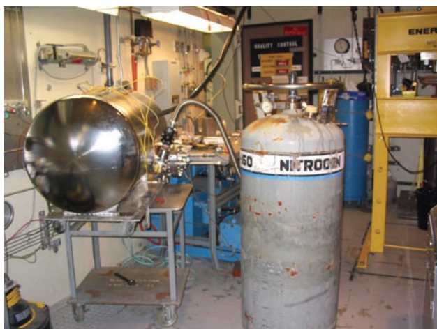
FIGURE 1. Cryogenic Testing of Vessel in LLNL High-Pressure Laboratory
