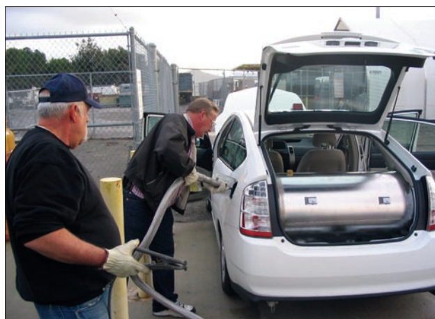
FIGURE 3. Prius Prototype Vehicle Being Refueled With Liquid Hydrogen at LLNL Fueling Station
