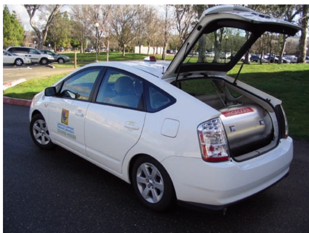
FIGURE 2. Cryo-Compressed Vessel Installed Onboard the Prius Hydrogen Fueled Hybrid Vehicle
