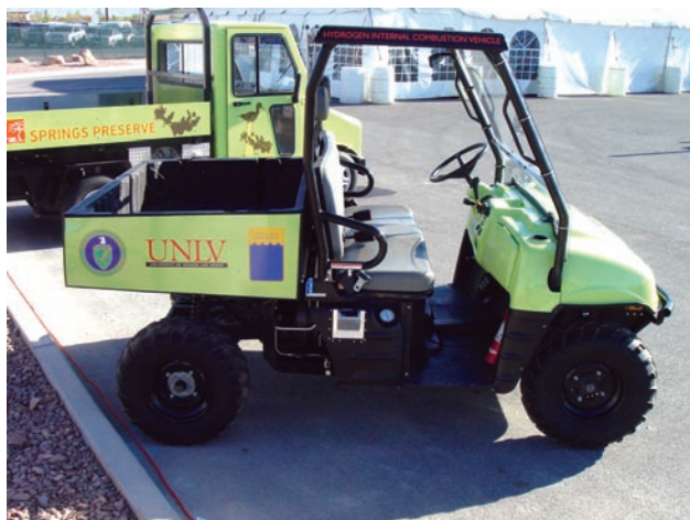
FIGURE 3. Polaris Ranger Hydrogen ICE Vehicle Shown with the Taylor-Dunn Fuel Cell Vehicle Shown in the Background
