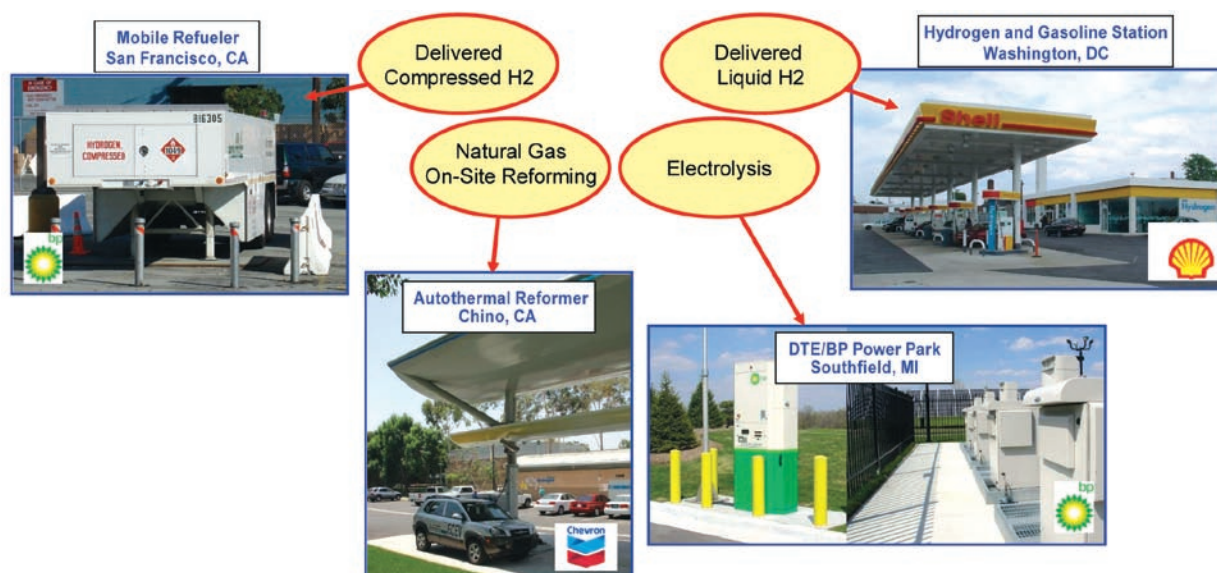
FIGURE 1. Four Types of Hydrogen Refueling Stations Being Tested
