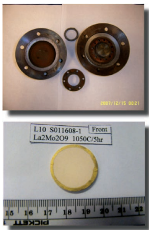
FIGURE 7. (top) UC hydrogen permeation cell with stainless steel components and graphite gasket for gas-tight seal; (bottom) 1-inch diameter fully-dense LAMOX ceramic with integrated gold seal around perimeter to minimize gas leakage.
