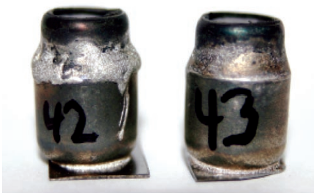
FIGURE 1. Successful Braze of Membrane Alloy to Stainless Steel
