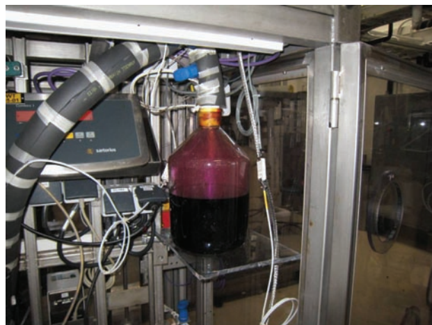
FIGURE 2. HIx Collected in Skid 1 at the Exit of the Bunsen Reactor
