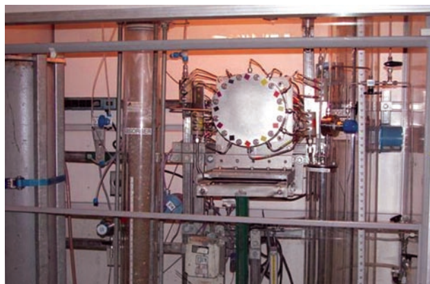
FIGURE 4. Photograph of Multi-Cell SDE Stack Installed in Test Facility
