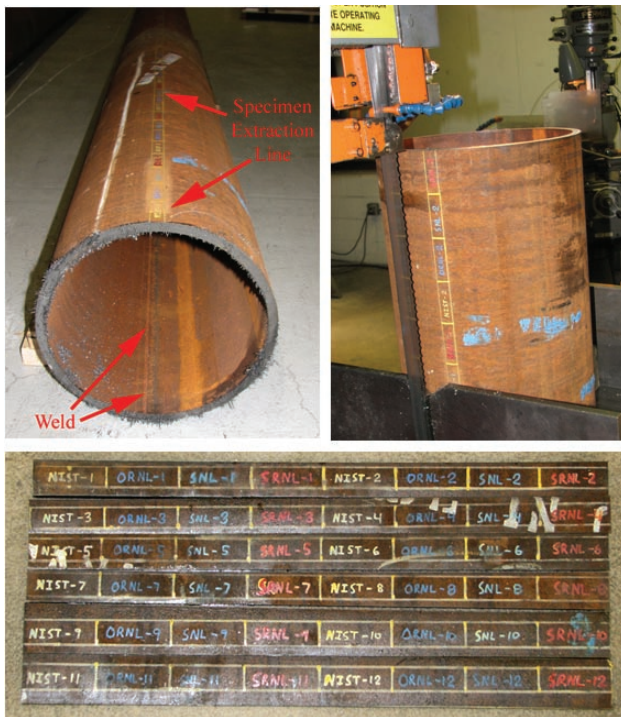
FIGURE 4. Fracture Toughness Specimen Tested in Air
