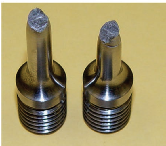
Hydrogen Faceted fracture surface with evidence for multiple secondary cracking, does not seem as severe as in Alloy A
