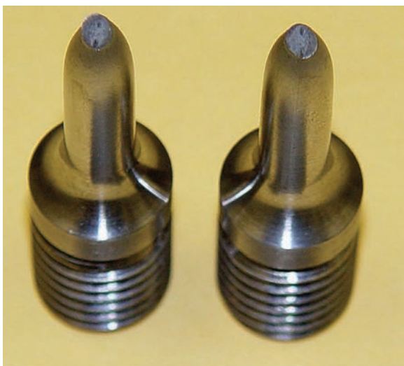
Helium Typical Ductile cup and cone fracture
