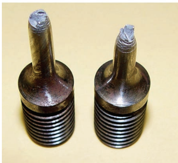
Hydrogen Faceted fracture surface with evidence for multiple secondary cracking
