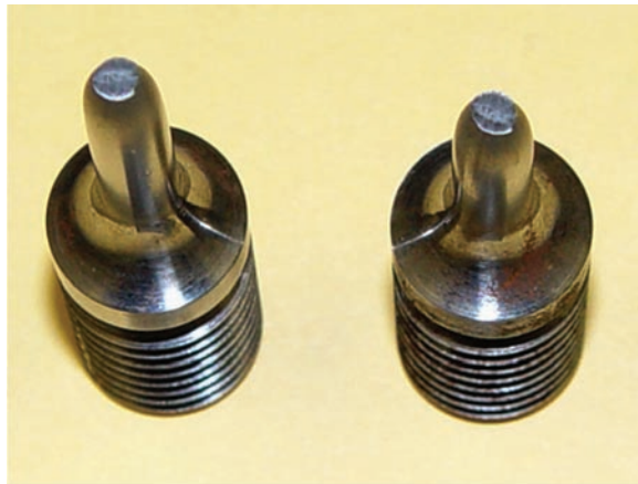
Helium Typical Ductile cup and cone fracture
