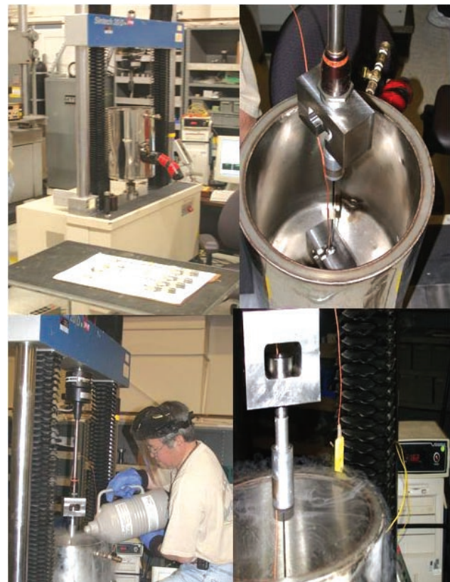
FIGURE 3. Experimental apparatus and procedure for testing campaign that broke pultruded glass fiber (basalt) composite specimens. Testing to failure occurred under pure uni-axial tension at constant (liquid nitrogen and ambient) temperatures, but uncontrolled atmosphere. Upper left: liquid nitrogen Dewar mounted into tension testing machine. Upper right: basalt rod mounted inside Dewar with invar fixtures into tension test machine. Lower left: Operator filling Dewar with liquid nitrogen in preparation for tension test. Lower right: Temperature stabilization in the basalt rod ahead of the tension test.
