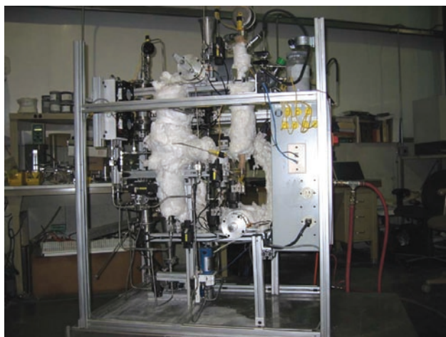
FIGURE 2. Mixer Showing Reactor and Pumps
