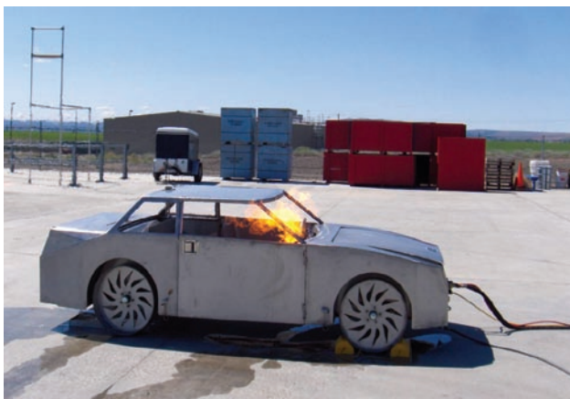
FIGURE 2. FCV Simulator Prop (The FCV simulator prop demonstrates potential conditions that could be encountered during the control and suppression of a FCV fire. The prop is being integrated into a training course, Hydrogen Safety for First Responders, being developed by PNNL and the Volpentest HAMMER Training and Education Center for the U.S. Department of Energy. The photo shows a propane flame that simulates a compartment fire.)
