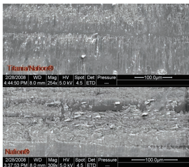
FIGURE 3. SEM micrograph of Nafion ® (bottom) and Nafion ® /titania (top) membrane after contractile stress buildup vs. time at constant strain experiments with drop in RH.
